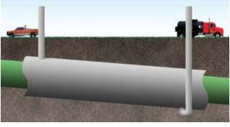
A top vent on the higher end of the casing and bottom vent on the lower end is ideal.
